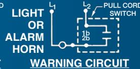
**NOTE:** Two circuit double break switches must be wired to equal voltage sources and the same polarity. Loads should be on the same side of the lines. 1B has the same polarity as 3A.
